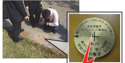
RFID installed benchmark, Nagareyama, Chiba
